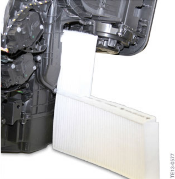
Heating and air-conditioning unit, replacement of microfilter
